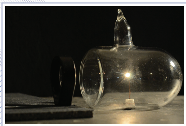
White-light emission from graphene and spectral intensity induced by focused infrared laser.
